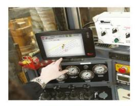
**Drill** can measure what the human eye can't, enabling your operators to drill accurately in the right position and to the correct RL the first time, every time. Accurate, high precision GPS navigation, coupled with real-time sensor feedback empowers site personnel to make informed decisions on management, production performance, operator performance, planning and consumables.
